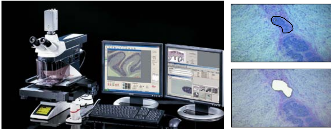
Figure: Laser capture microscope (left). The particular area of cancer cells shown in the right upper image has been “cut out” by laser microdissection for analysis (right lower image).
